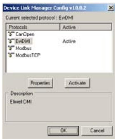
For **Smart** select **EwDMI** or **Modbus**<sup>[2]</sup>. If the protocol is not activated press the **Activate button**
