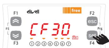
The first parameter shown is CF30. To view the value of the parameter press the set key.
