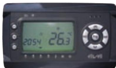
**SKP22 remote terminal with LCD display without backlighting**
