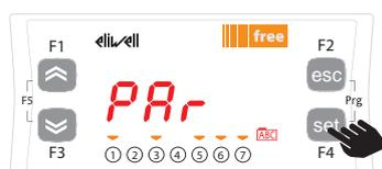
The parameters menu PAr contains all controller folders. Press the set key to view folders.
