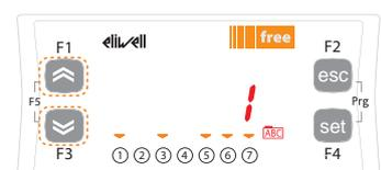
Use the UP and DOWN keys to change the value if necessary. To confirm the value press the set key. To exit press Esc
