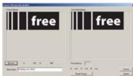
We recommend that you import black/white images of suitable size. The display can support an image of approximately 100x50px. The imported bitmap will be in the **Bitmaps node**<sup>17</sup>
