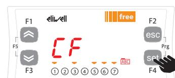
The first folder shown is the CF configuration folder. Press the set key to view the folder parameters.
