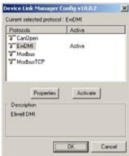
Also in this case, the properties are visible and can be edited from the panel **Communication > Settings > Properties** **Communication > Settings > Properties**<sup>[7]</sup>. The panel displayed depends on which protocol is activated:
